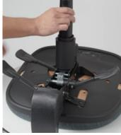
6. Insert the new gaslift into the hole in the metal mechanism.
