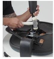
4. Hold the gaslift while striking the metal mechanism around the point where the gaslift enters. The gaslift should pull out easily.
