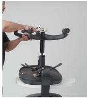
3. Strike the rim of the bottom of the gaslift firmly with a hammer and pull the 5-star base upwards and off the gaslift.
